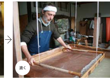
漉く 漉き舟に水と紙料、ネリを入れて均等に整えたと、漉く Add pulp, water and neri to the vat and scoop up into a screen in the nagashisuki method
