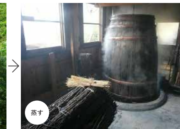
蒸す 刈り取った原木を1m程に揃え、薪のカマドで蒸す Steaming the harvested pieces of pulpwood, which are cut to a length of one meter, on a wood-fired stove
